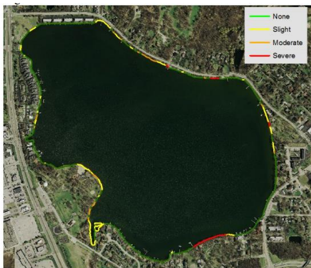
Figure 44: Lake Zurich Shoreline Erosion Condition, 2015
