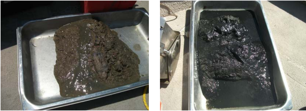
Figures 30 & 31: Sediment near the dam is much lighter in color than in the northern section of the lake. The light colored soil typically represents agricultural deposition.
