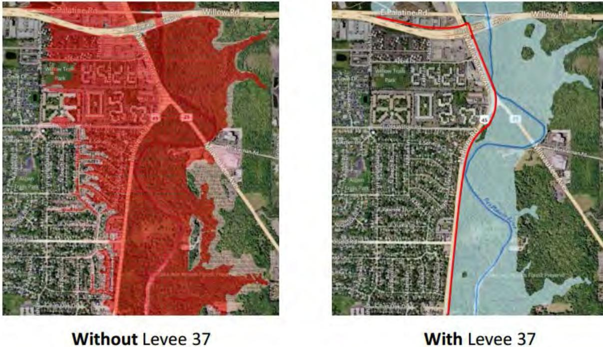
**Figure 4-13: Potential Flooding with and without Levee 37. Images courtesy of MWRD.**
