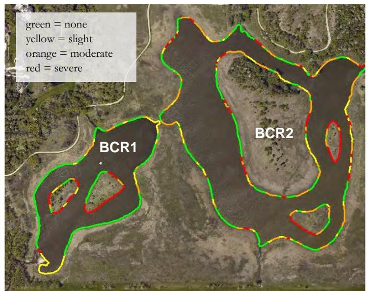
**Figure 3-50: Shoreline Erosion on Buffalo Creek Reservoir, 2013.**
