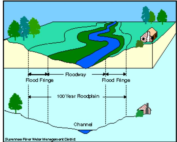
**Figure 4-1: Graphic of a Typical Floodplain. Source: Suwannee River Water Management District.**
