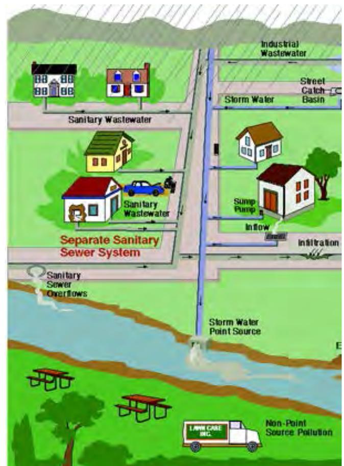
**Figure 5-10: Municipal Storm Sewer System.** Source: [http://www.epa.ohio.gov/portals/35/cso/wet\\_weather\\_flow\\_graphic.jpg](http://www.epa.ohio.gov/portals/35/cso/wet_weather_flow_graphic.jpg)
