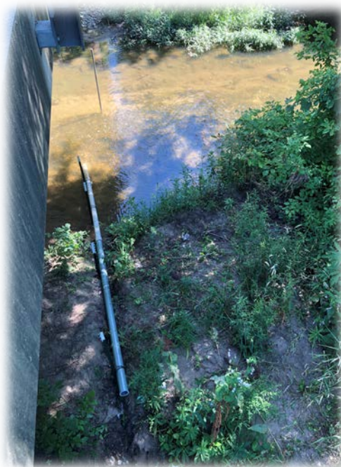
Example of Sensor Deployment: sensor placed inside PVC pipe and anchored to stream
