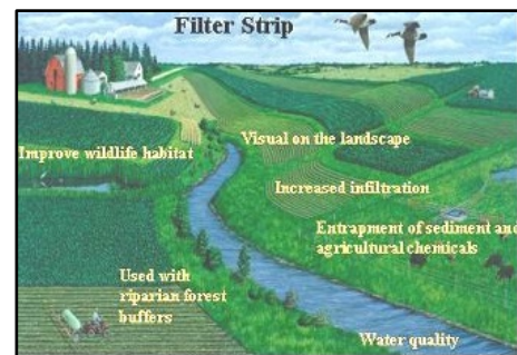
Schematic of a filter strip and illustration of its benefits (USEPA 2017).
