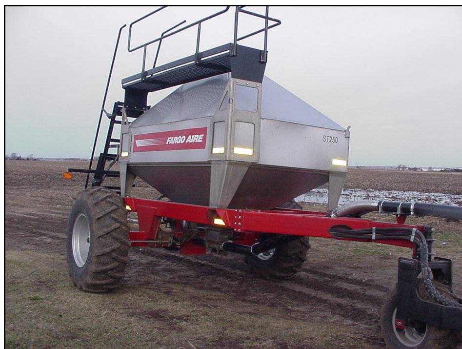
Figure 4-1. Deep Placement Phosphorus Attachment Unit for Strip-till Toolbar.
