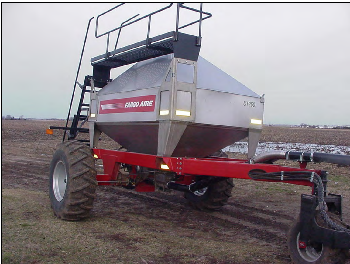
Figure 4-2. Deep Placement Phosphorus Attachment Unit for Strip-till Toolbar.
