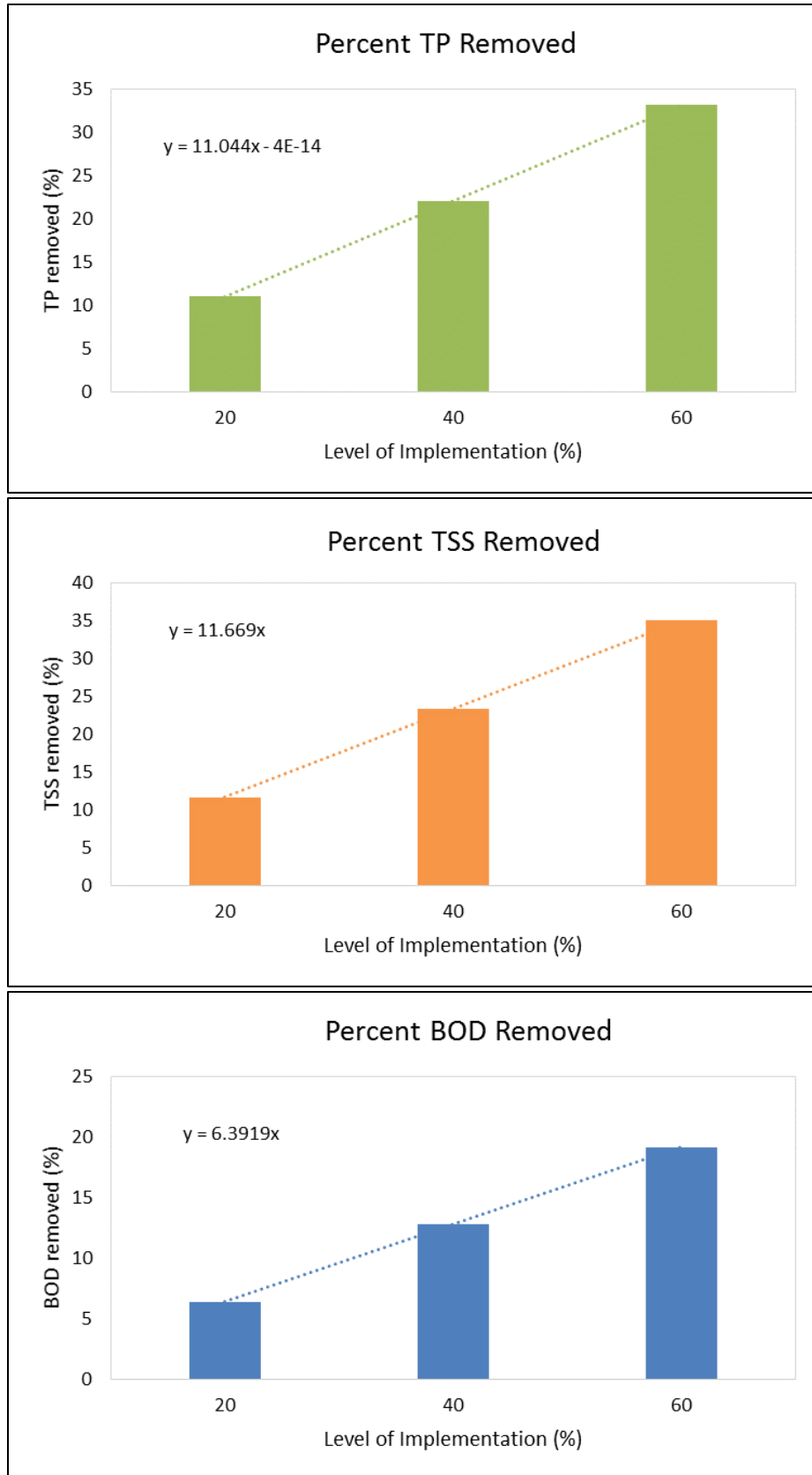
Figure 80. Implementation curves, West Branch DuPage River subwatershed.
