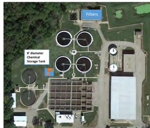
Figure 17 – Site Plan for Chemical Phosphorus Removal
