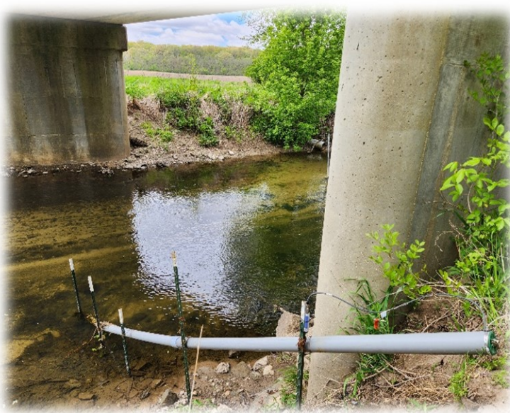
Station RCDC at the Hays Ave. Bridge Showing Temporary/Passive Deployment of Monitoring Infrastructure
