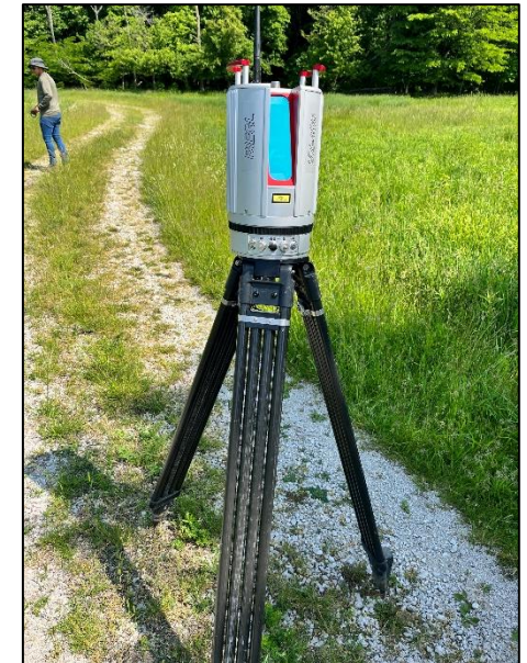
LiDAR scans to reveal channel bank migration
