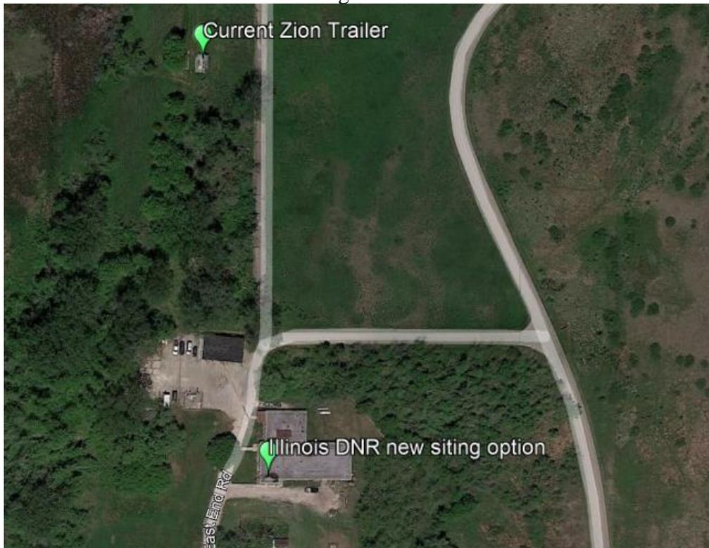
Champaign: USEPA approved a site move across the street for the Champaign PM2.5 monitoring site. The new location is better suited for power and a transition to continuous FEM monitoring. The AQS site identifier is unchanged and GPS coordinates have been updated. This change took place Q2 2024. Figure 2 below illustrates the move.
