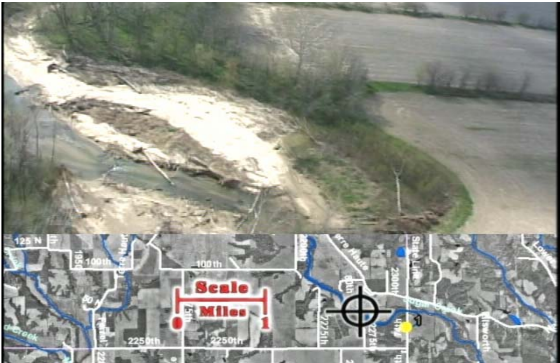
Fig. 5 Channel changes due to large sand deposits and lateral erosion (Chapter 1)
