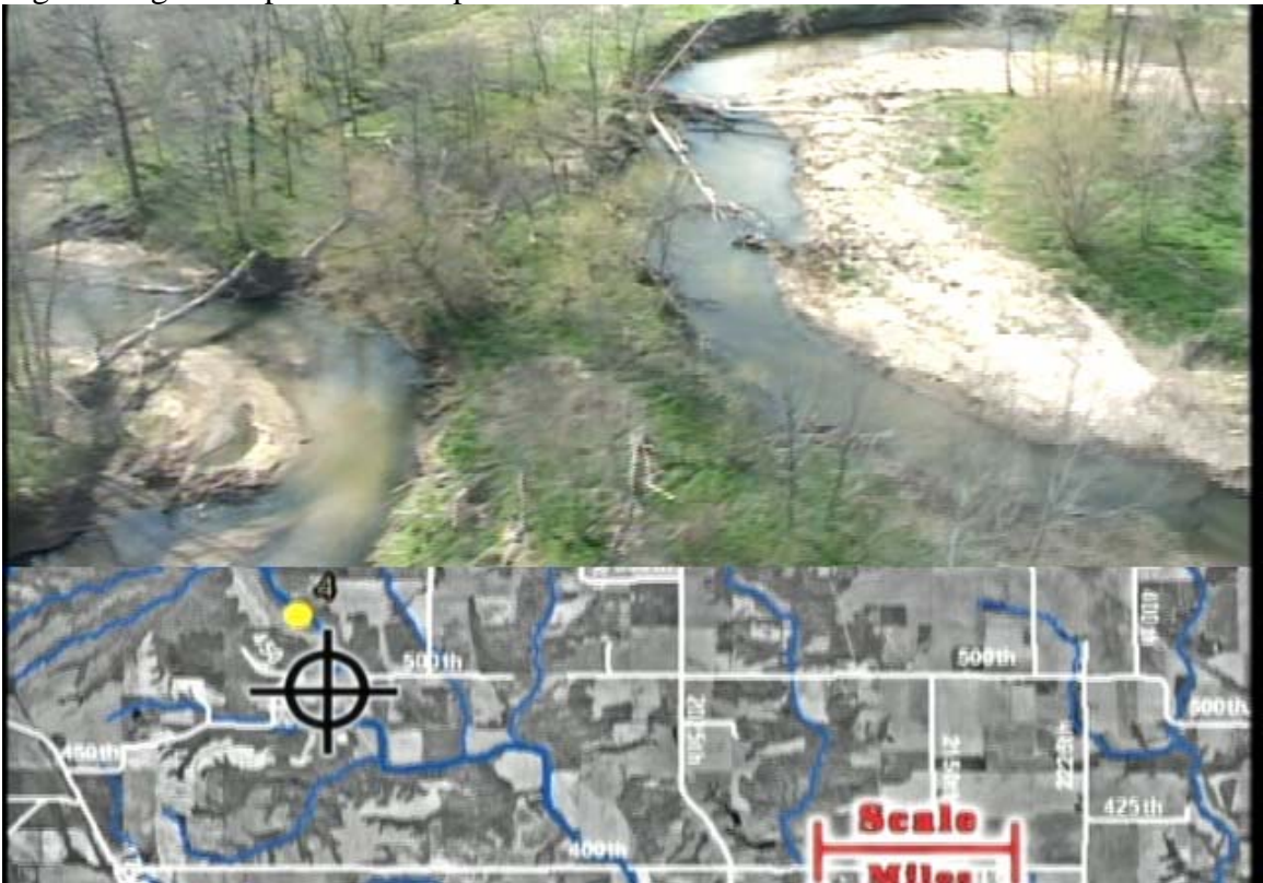
Fig. 10 Downstream lateral migration resulting in unstable planform and eminent cutoffs
