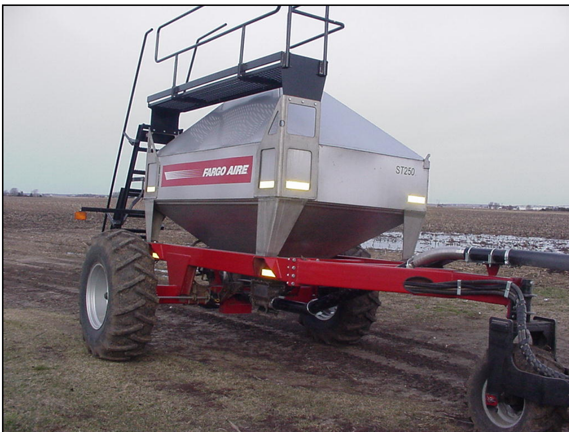
Figure 4-3. Deep Placement Phosphorus Attachment Unit for Strip-till Toolbar.
