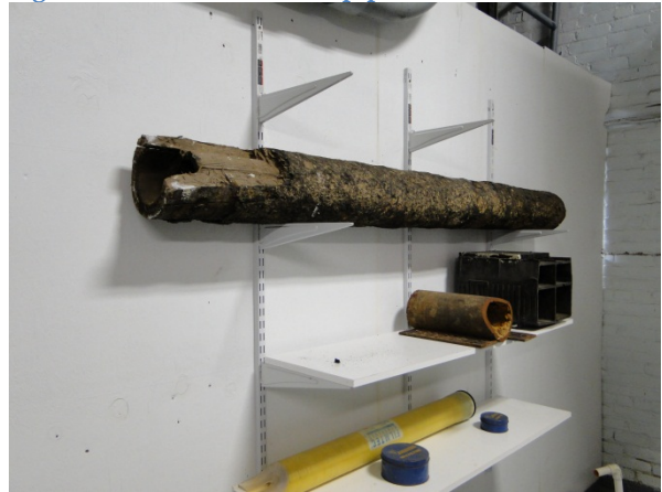
Figure 18. Old wood water pipe from Macomb
