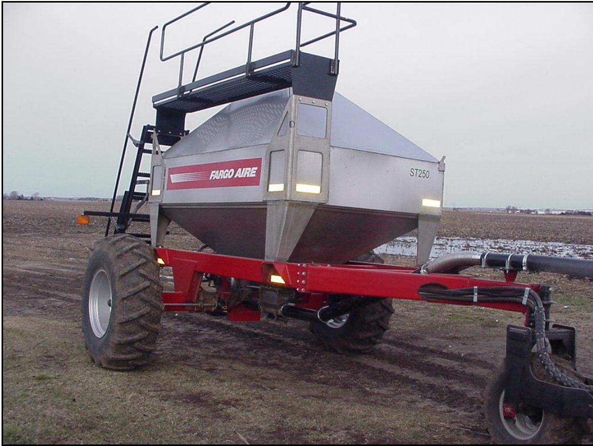
Figure 5-3. Deep Placement Phosphorus Attachment Unit for Strip-till Toolbar.
