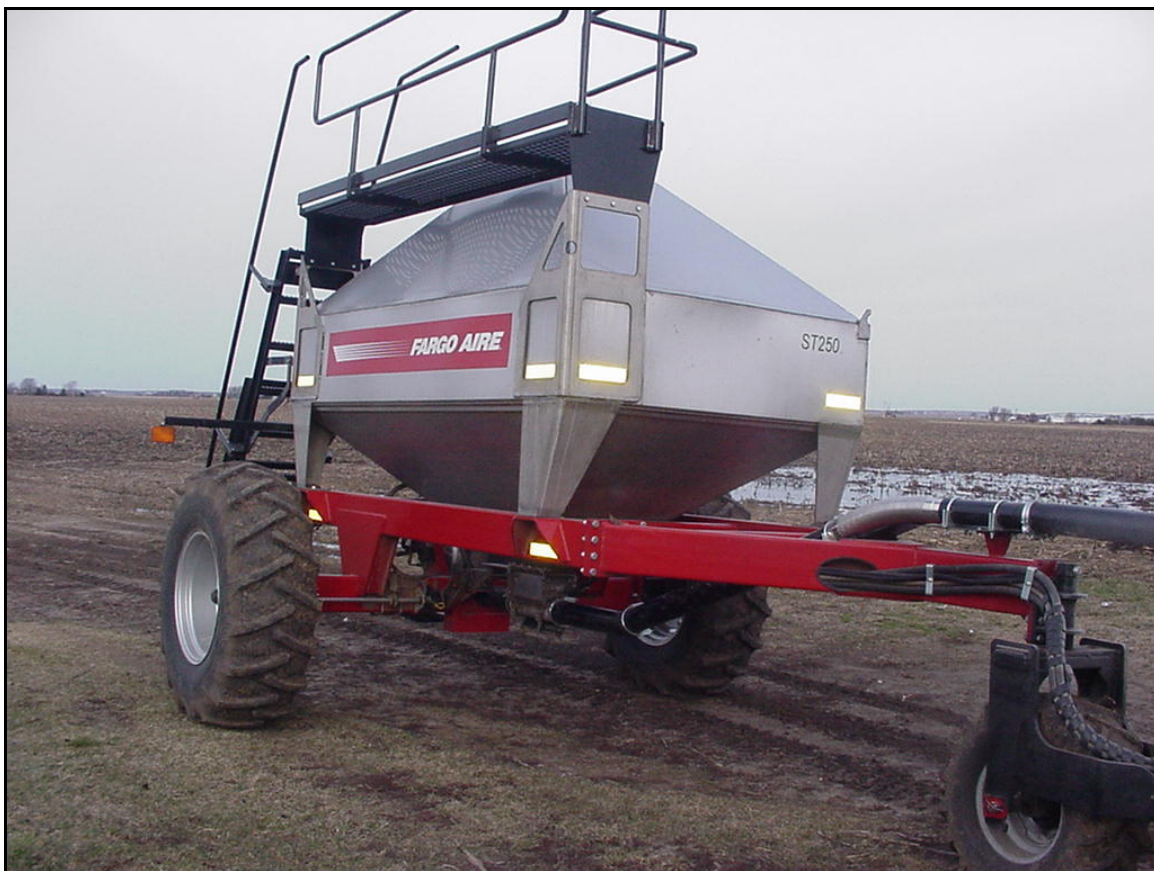
Figure 5-1. Deep Placement Phosphorus Attachment Unit for Strip-till Toolbar.
