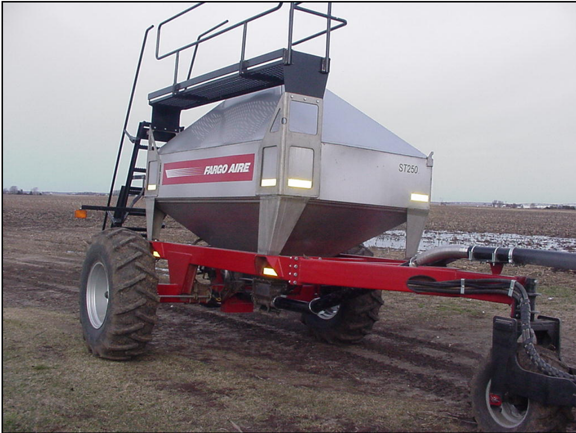
Figure 4-13. Deep Placement Phosphorus Attachment Unit for Strip-till Toolbar.
