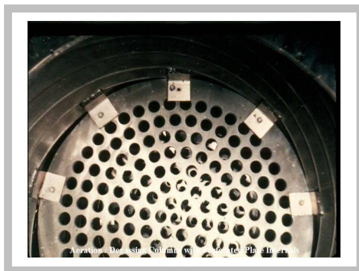
Figure 5-4 - Diffuser Used for Bubble Aeration
