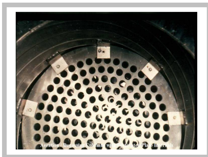
Figure 6-4 - Diffuser Used for Bubble Aeration
