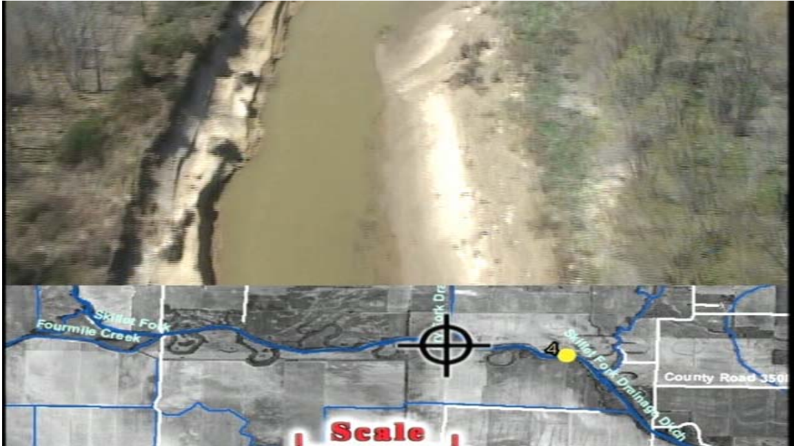
Fig. 25 Severe erosion below active knickzone at 40:37 on DVD disc 1.
