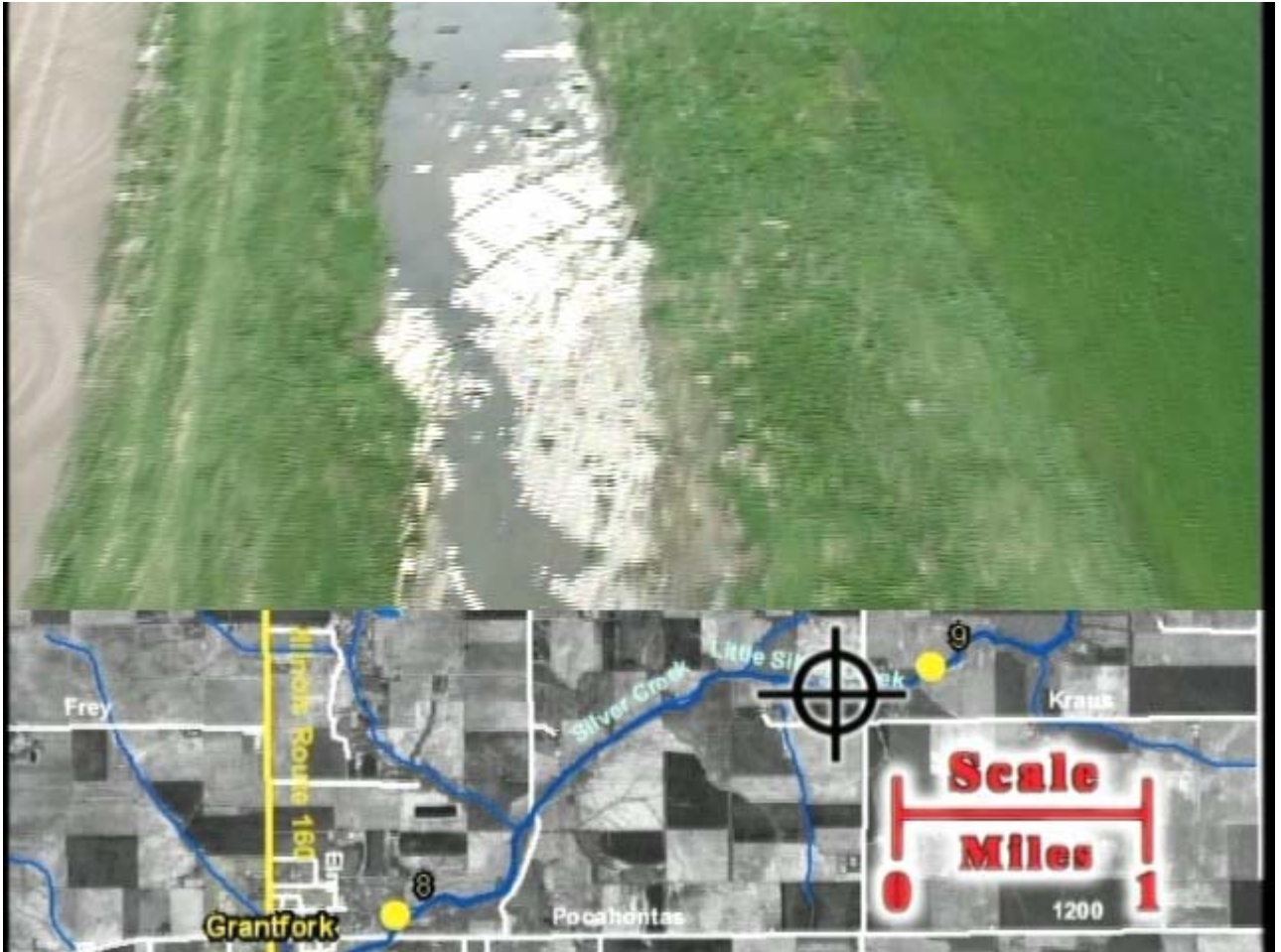
Figure 6: Captured image showing bedrock channel bed from 43:41 min. to 44:00 min. on DVD. Note bank stability in the area of bedrock grade control.
