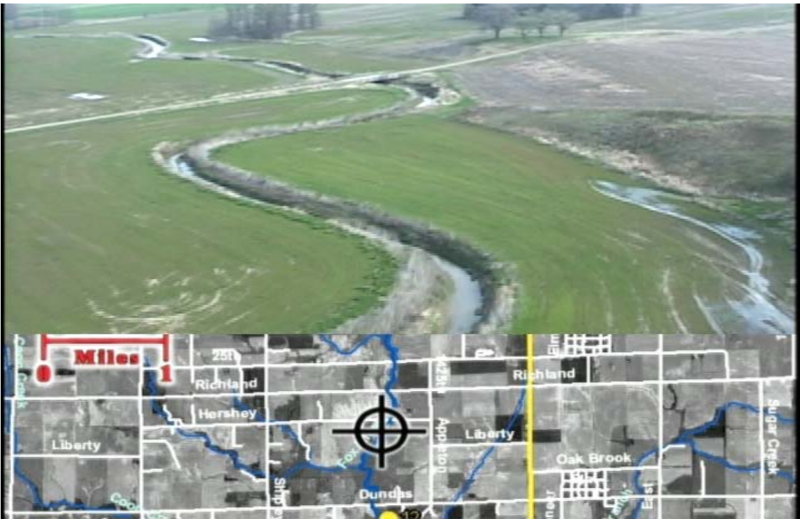
Figure 13 Channel segment with riparian border removed—but little or no straightening: DVD Tape 2 at 27:14
