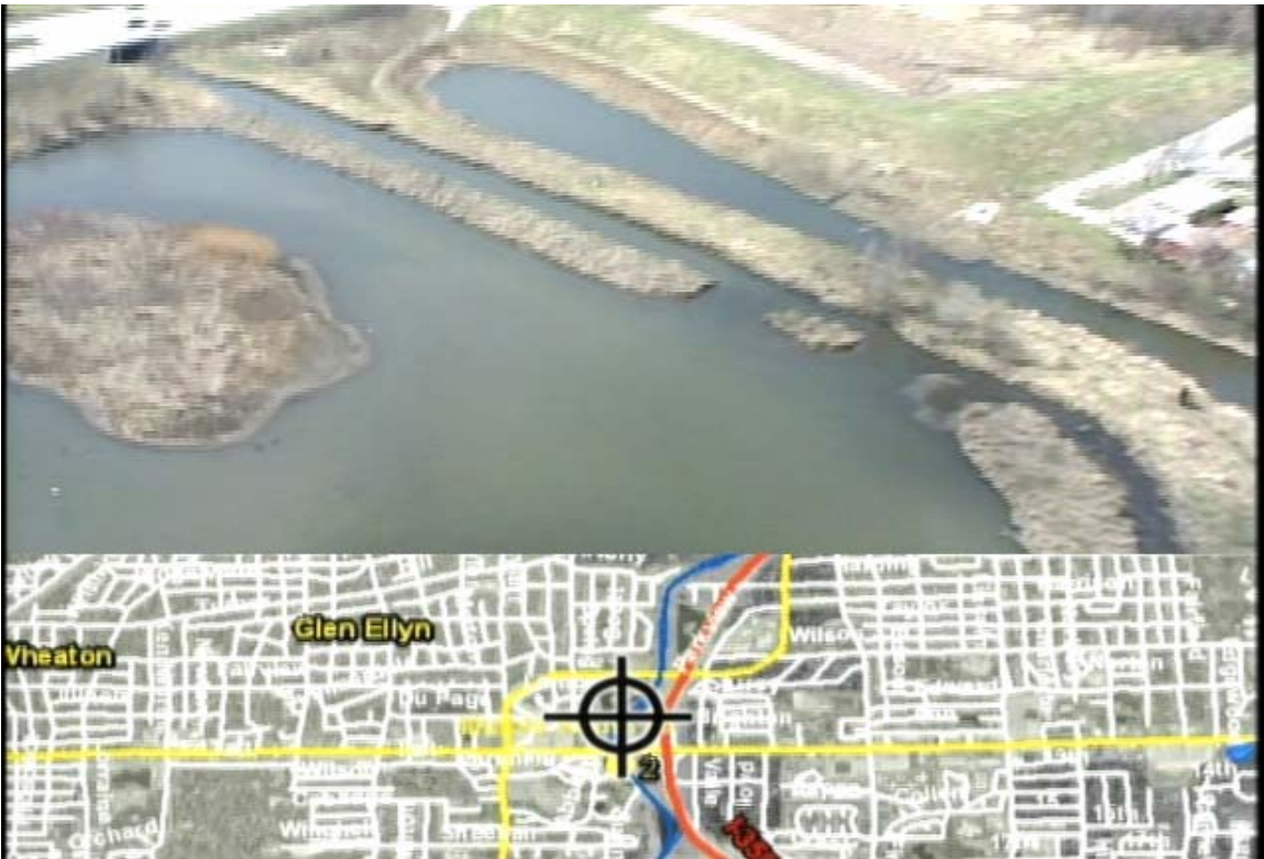
Fig. 8 Exit breach back into “old channel”
