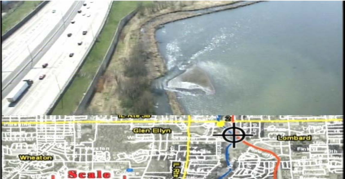
Fig. 9 Lake below IL. Rte. 38 where East Branch has again breached levee with similar results.
