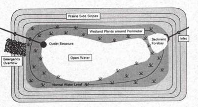
The detention pond's depth influences its water quality. Generally, detention ponds should be deep enough to maintain open water areas and limit sediment resuspension by current, wind, or waves. Typically, the average depth should be at least 4-5 feet and maximum depth at least 8 feet. If you want fish to survive through the winter, it is generally recommended that at least 25% of the pond be at least 10-12 feet deep.
