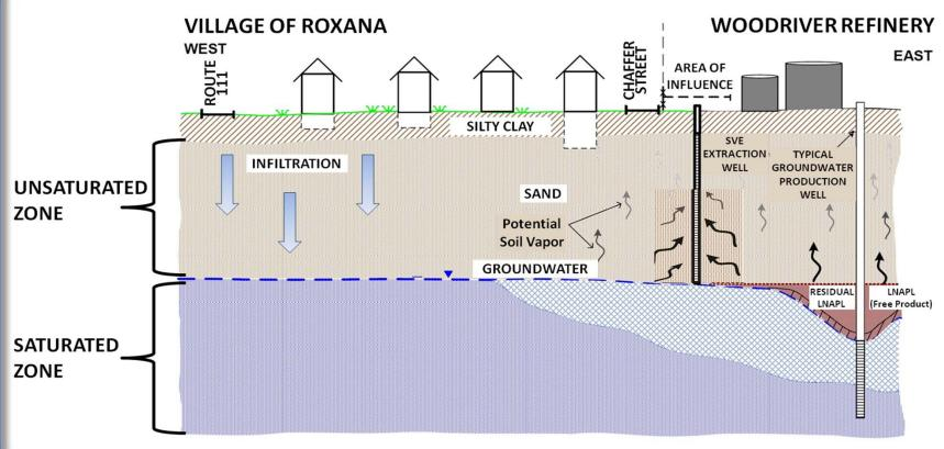
**Free Product measured in Roxana** is a result of historically released petroleum products and has been measured in 3 groundwater monitoring wells in Roxana. These products are lighter than groundwater so they will typically be found near the top of the groundwater.
