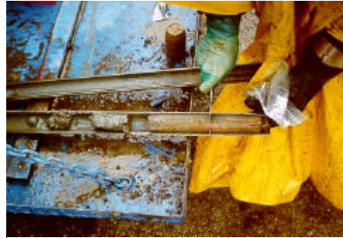
Core sampling to determine extent of contamination
