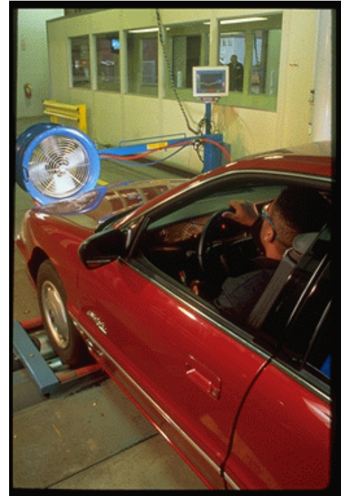
The new vehicle emissions test will include a dynamometer (treadmill) test.
