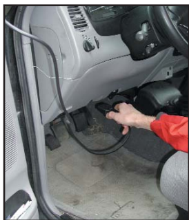
On Board Diagnostics (OBD) testing is done by connecting to the vehicle's on board computer and retrieving information about the vehicle's emission control equipment.
