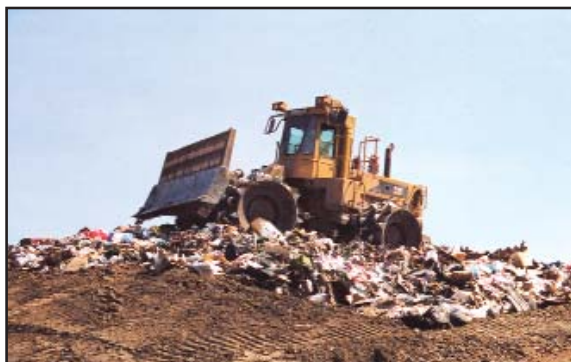
Compaction and spreading of garbage at a municipal waste landfill
