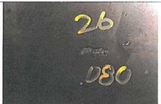
Description: Arc gouged area at tray level 26. .080 x 1.5"
